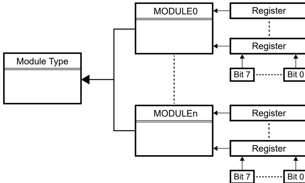
A module type can be the Universal Synchronous-Asynchronous Receiver Transmitter (USART), while the module instance is, e.g., USART0, where the 0 suffix indicates the instance is "USART number 0". For simplicity, a module instance will be referred to as a module throughout this document, unless there is a need to differentiate.
