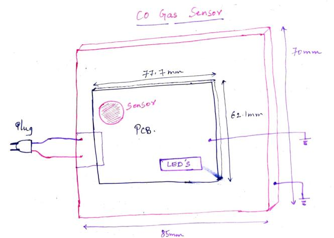
\* Aluminium Casing is incorporated and surface is earthed.
