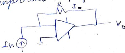
In the figure shown above, the current  $I_{in}$  is the one from sensor which is given as input to an Op-amp. The feedback resistor ~~which~~ will have a drop of  $I_{out} \times R$  which will be same as  $V_o$  ( $V_o = -I_{out} R$ ) (Due to virtual ground concept,  $I_{in} = I_{out}$ ) So now voltage is obtained but the next stage will also be a voltage det detection of fault voltage using Op-amp.
