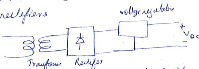
Use of transformers makes it bulkier and can lead to electromagnetic interference issues, makes it costly.
